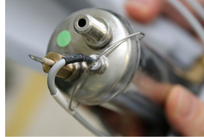
There is a SONTEC NTC plug-in sensor in the compact hot water boiler that registers the current water temperature with a fast response time of T05 within 1.5 seconds.
