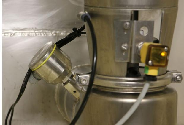
Thanks to optimised flow geometry and very fast response times the ICS-8 is ideal for phase separation, product detection and measurement of media concentration in CIP plants.
