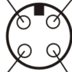
D1: M12 Stecker 4pol, MU Pin 1(+), Pin4 (4-20 mA), Pin 2+3nc
