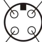
D2: M12 Stecker 4pol, MU Pin 1(+), Pin3 (4-20 mA), Pin 2+4nc
